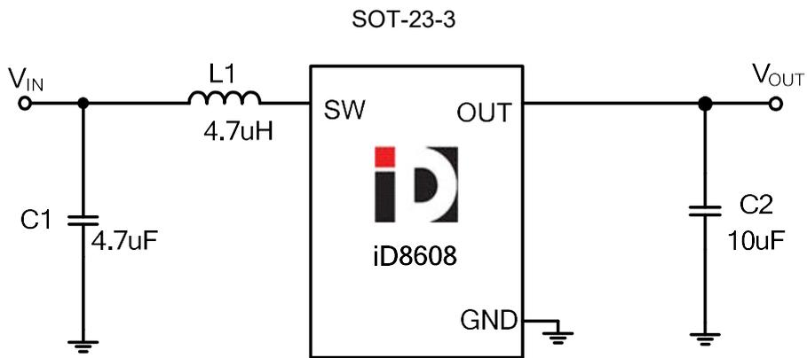
**Option Application Circuit (Output Fix 3.3V)**
